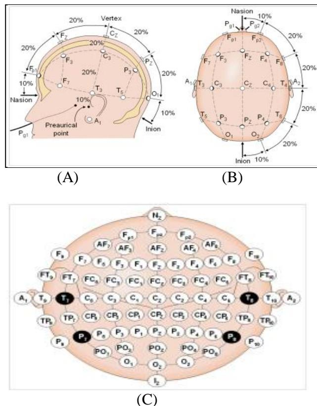
Figure1: Electrode Placement
