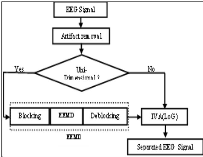
Figure 2. Flowchart of existing and proposed algorithm.
