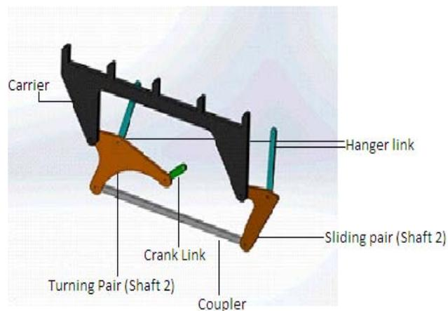
Fig: 4.1. Design of Main Frame
