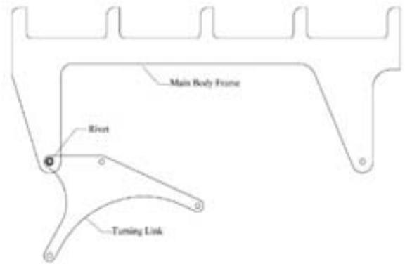
This is a second step for sub-assembling of metal body frame. In this sub assembling Turning Link is connected to left side of the main body frame by using rivet and while assemble we should maintain some gap between this two links for a free movement turning link this gap maintain with the help of bush. Here, we use “loose running fit” between links.
