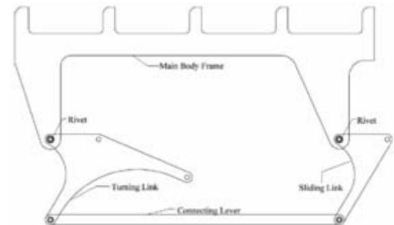
This is the third step for sub-assembling of metal body frame. In this assembly, sliding link is connected to right of the main body frame by using rivet and we also maintain some gap between these two links for free movement of sliding link when it slides over the main body frame this gap maintain with the help of bush. Here we should maintain equal gap between turning link (shaft 1), sliding link (shaft 2) and main body frame (carrier). We use “loose running fit” between links.
