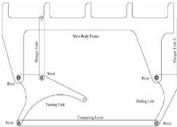
This is fifth step for sub-assembling of metal body frame. In this assemble, two hanger links are connected to right of the sliding link as well as right side of the turning link by using rivet and we also maintain some gap between this links for free movement of links and other side of this hanger are connected to wood frame 1.
