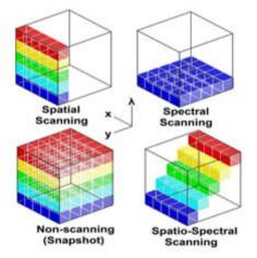
Fig. 4 Technologies for Hyperspectral Data Acquisition[8]
